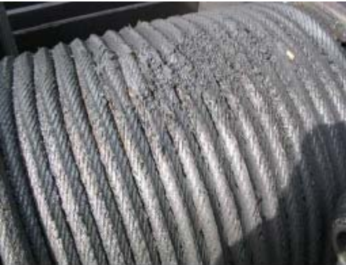
Wire rope showing crushing damage
