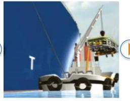
ROV operator on-board support vessel guides ROV HullWiper to approach ship and once in position engages cleaning mechanism.
