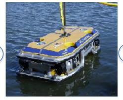
Removed fouling is captured on-board the HullWiper's fouling retrieval units and only clean water is released back into sea. Process is monitored during the whole cleaning operation.
